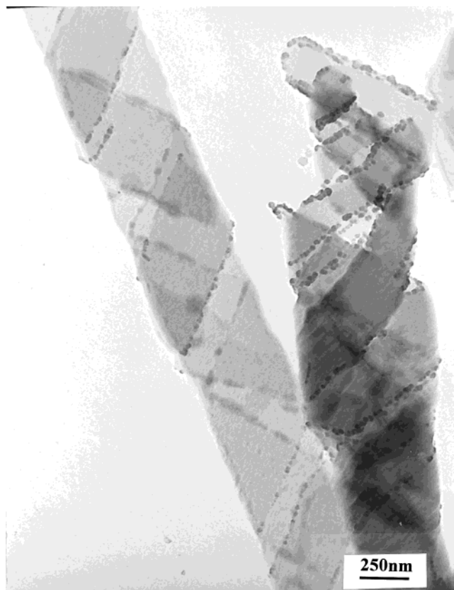
Figure 2. Separated beads of Ppy on a tubule. Note the separated beads on the tubule edges, with diameters ranging from 10 to 20 nm. The lipid ribbon (helix) that covers the closed tubule on the left-hand side of the image has been decorated along both its edges by Ppy. Polymerization conditions: 5 mM (\text{NH}_4)_2\text{S}_2\text{O}_8 , 0.02 M py and 8 mM \text{DC}_{8,9}\text{PC} in Millipore water, 15 min.
